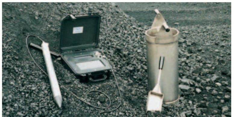
*Probe and Display Unit with calibration equipment.*
